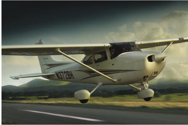
Figure 6-37. The landing gear supports the airplane during the takeoff run, landing, taxiing, and when parked.
