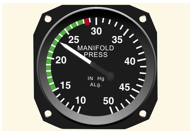
Figure 6-9. Engine power output is indicated on the manifold pressure gauge.
