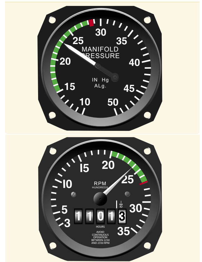
Figure 8-4. Manifold pressure gauge (top) and tachometer (bottom).
