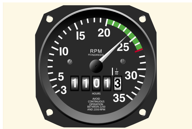
Figure 6-8. Engine rpm is indicated on the tachometer.
