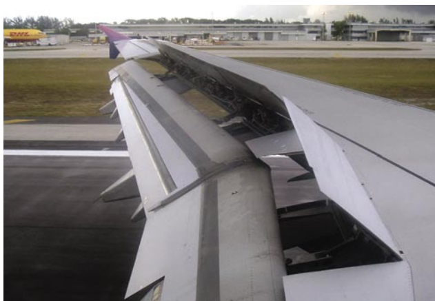
Figure 5-19. Spoilers reduce lift and increase drag during descent and landing.
