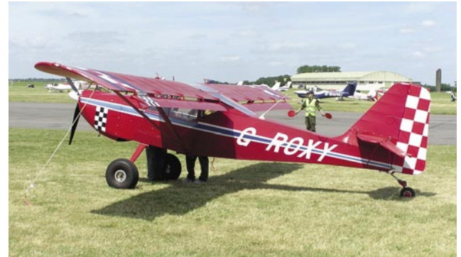
Figure 5-9. Flaperons on a Skystar Kitfox MK 7.
