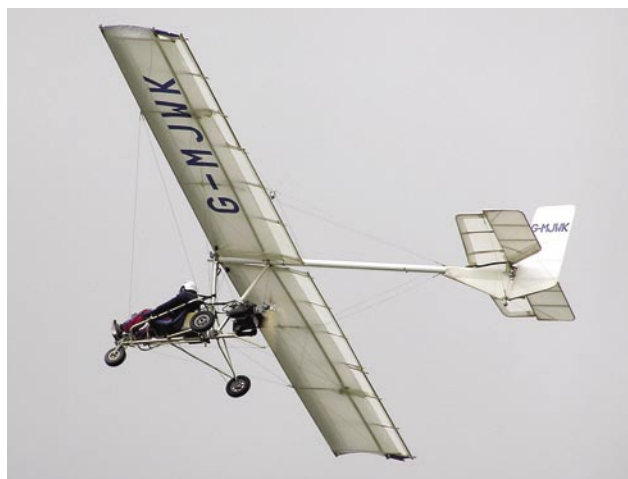
Figure 1-20. A typical ultralight vehicle, which weighs less than 254 pounds.
