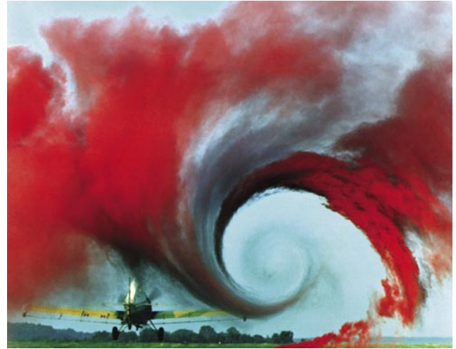
Figure 4-7. Wingtip vortex from a crop duster.
